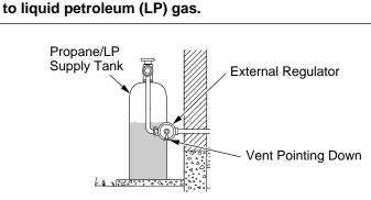
Figure 12 - External Regulator With Vent Pointing Down (propane/LP systems only)
